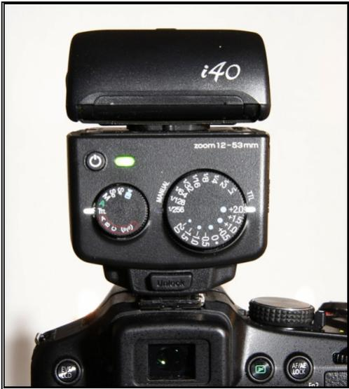
*TTL flash gun in TTL mode on the hot shoe*
