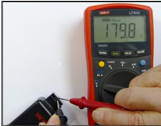
*Measuring the trigger voltage*
