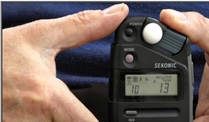
*The Sekonic L308S light meter for Flash and ambient metering.*
