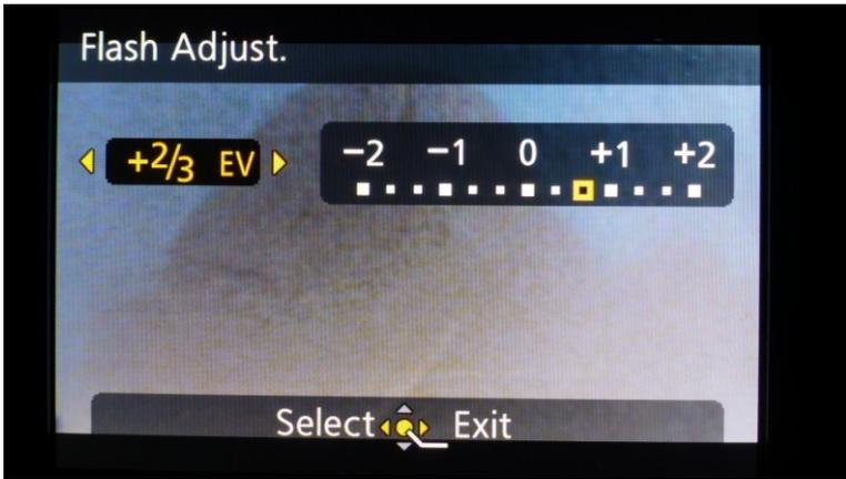
The flash power can be increased or reduced by the equivalent of 2 complete f-stops. This is a handy feature if you find the flash is consistently causing blown out or dark images.
