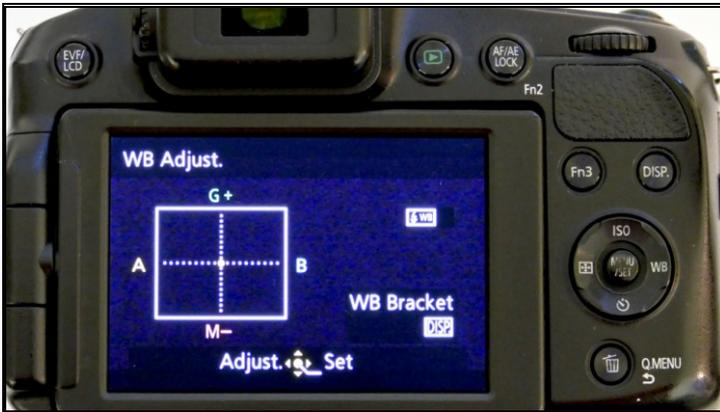
You can place the control points in any position between axis to change the overall colour of the change applied. For example placing the control in the lower left quadrant adds yellow and magenta which results in a red colour tint applied to the image.
