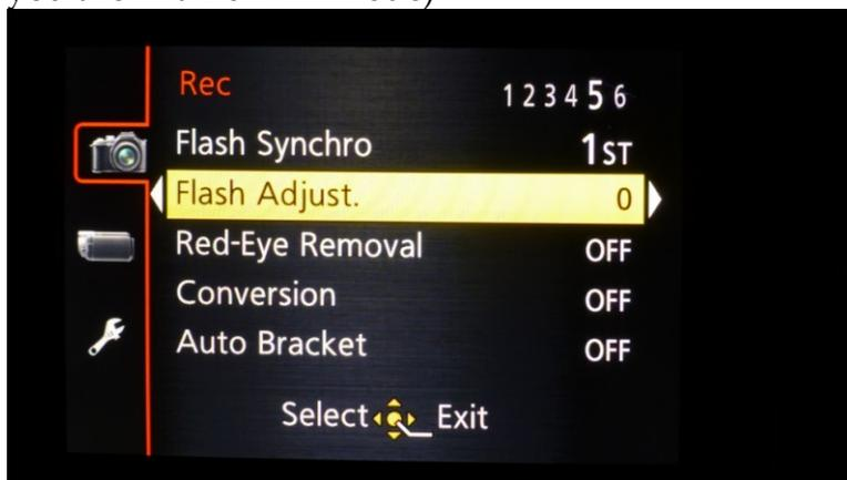
*Adjusting the power output of the flash setting.*
