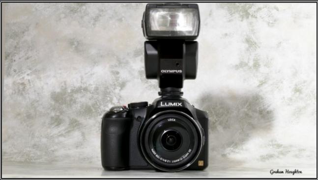
*TTL compatible flashgun inserted in the hot shoe*
