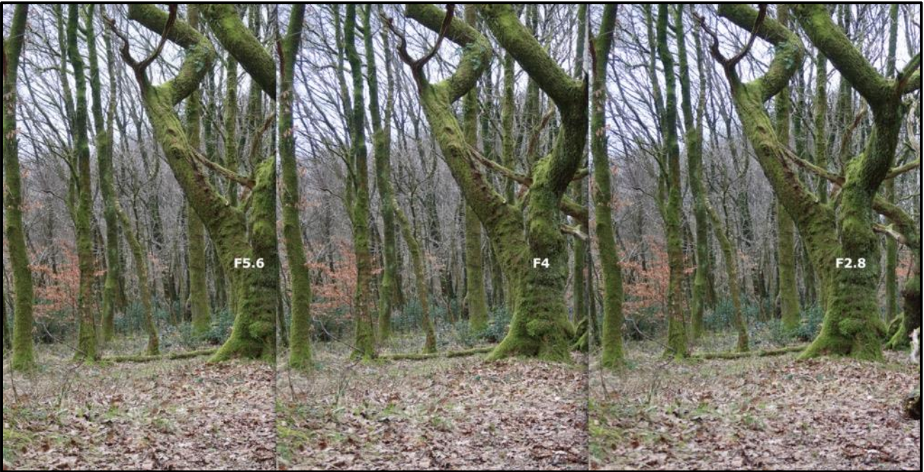
Establishing the point at which centre and edge definition are equal. At 50mm EFL F5.6 appears to be the sweet spot for this lens.
