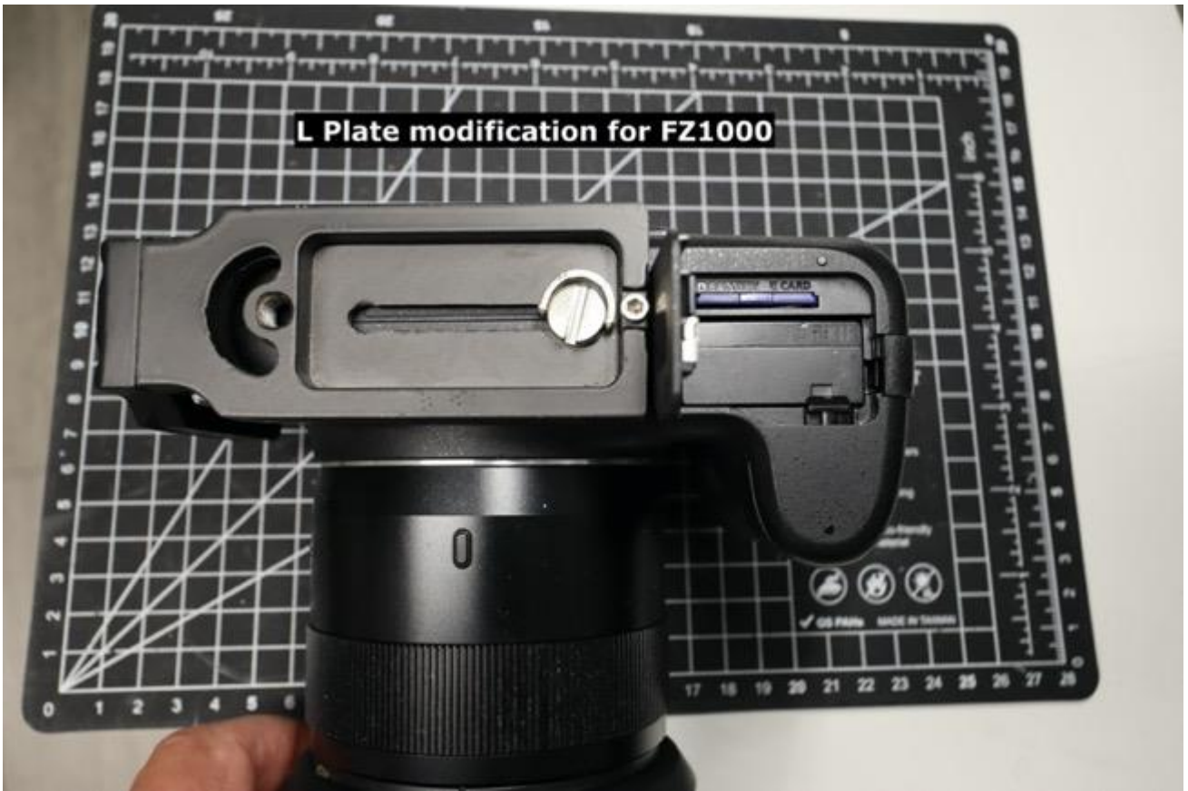
Showing the completed plate allowing access to the battery compartment
