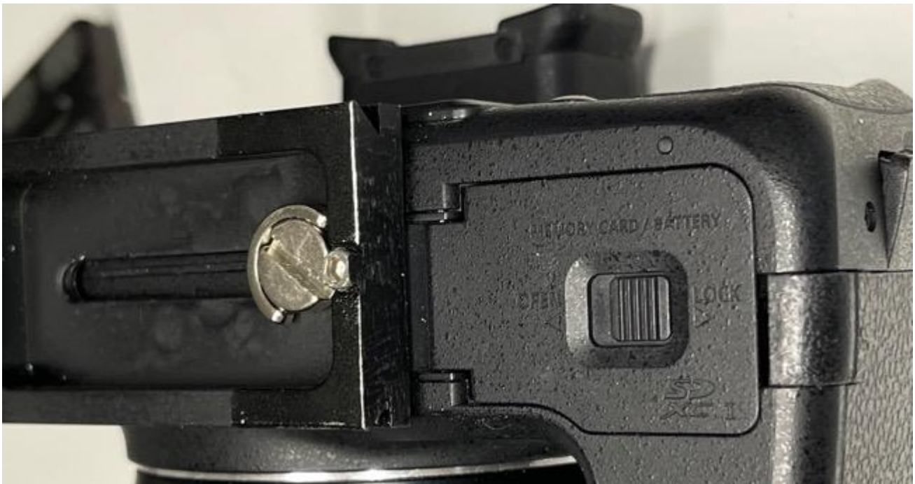
The finished plate milled and spray painted
