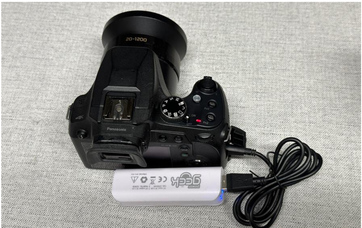
What I do is to occasionally plug the FZ80/82 into a USB charger to “top-up” the battery.
