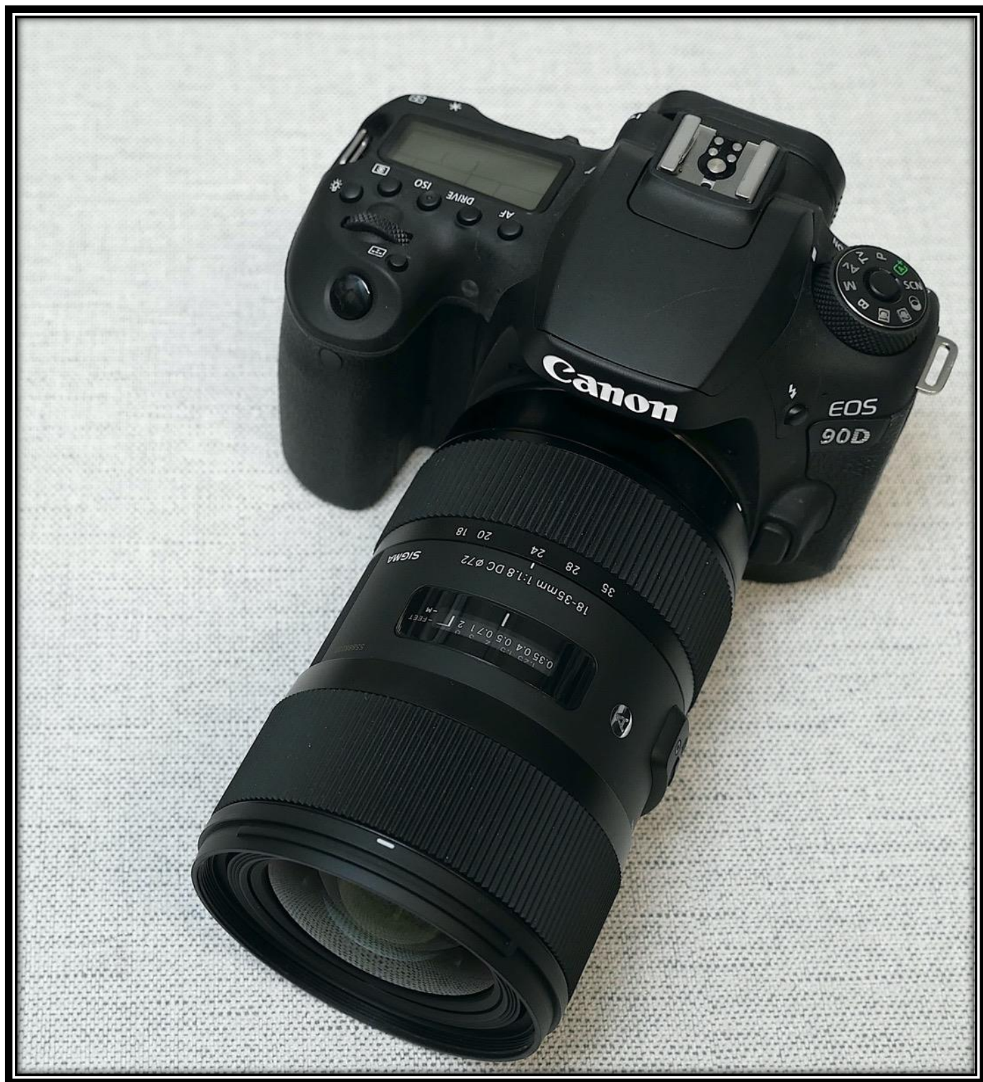
So this is the Sigma 18-35mm F1.8 Art lens fitted here to my Canon 90D DSLR camera.
