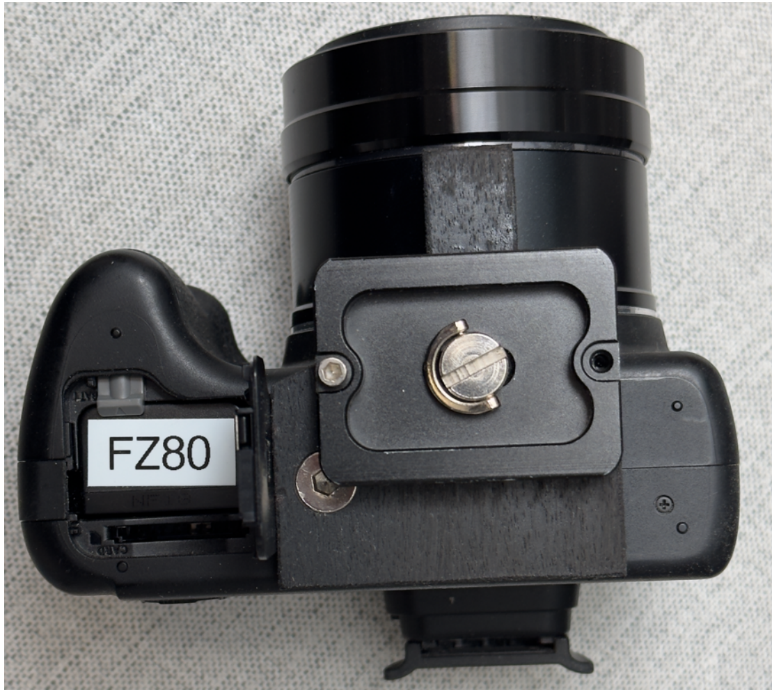
The final plate with a Arca style quick release plate attached allowing access to the battery and SD card compartment. The camera pivots now on the lens axis!
