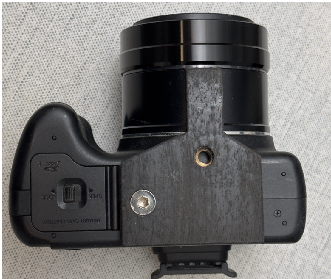
The plate attached to the camera with \frac{1}{4} -20 countersunk screw.
