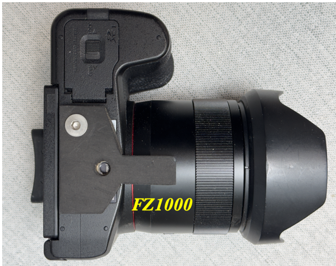
The final plate with a Arca style quick release plate attached allowing access to the battery and SD card compartment. The camera pivots now on the lens axis!
