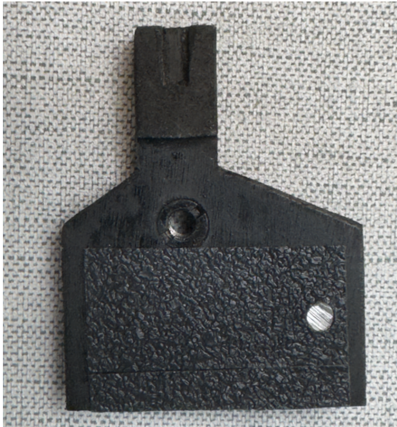
The rubber sheet attached on the upper surface.
