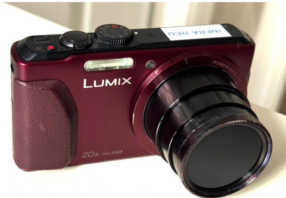
A later converted TZ40 with the 37mm 720nm IR Pass filter.
