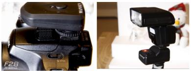
The wireless trigger and receiver on the flash unit
