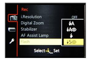
In this mode the shutter speed is set to a longer exposure time thus allowing more of the ambient light to affect the final exposure. It is useful for recording brighter background in your images rather than have the usual dark/black background we normally associate with flash pictures, especially outdoors. Again red eye reduction is employed during this exposure sequence.
