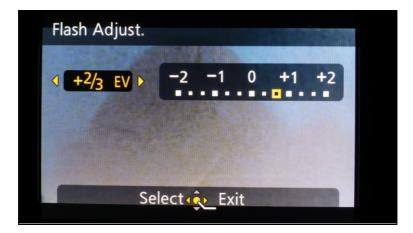
The flash power can be increased or reduced by the equivalent of 2 complete f-stops. This iA a handy feature if you find the flash is consistently causing blown out or dark images.
