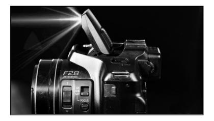
In the case of the Panasonic Lumix Bridge cameras the pop up flash provides only a direct on axis light source, and, unlike the later FZ1000 model cannot be used as a remote commander to control other external flash units either singularly, or in groups.
