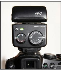
TTL flash gun in TTL mode on the hot shoe
