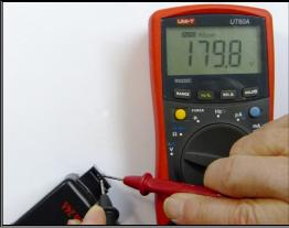
Measuring the trigger voltage
