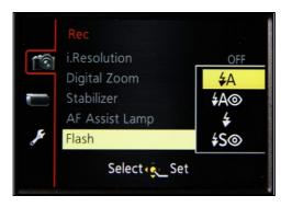
In this mode the camera determines if the flash is required (based upon ambient light) for the exposure, and, if it does so controls the amount of light required by monitoring the light captured by the sensor in a short pre-flash burst of light prior to the main exposure. It then adjusts the main flash pulse duration to control the exposure.
