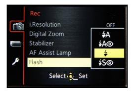
With forced flash set on the camera will fire the flash with every exposure irrespective of the ambient lighting conditions. This is useful if you are using the flash for fill in flash exposures where in the auto modes the flash would probably not fire in bright ambient light conditions. Again flash power can be set with the Flash Power adjustment menu.
