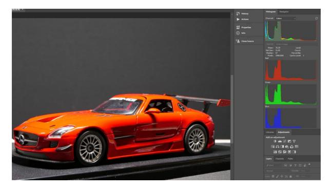
Note the red channel has a spike right at the red saturation (255) value
