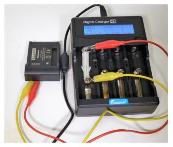
By utilising a commercial charging unit and the charging plate from a USB charger I could connect the charging terminals of the charger to the battery under test on the USB charging plate.
