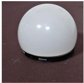
The opal diffuser glued to an old 52mm filter ring
