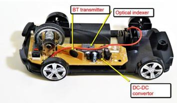
As the unit is powered by just 1 single AA battery I suspected that the unit must have some form of DC-DC convertor (like a Joule thief circuit) to power the RF transmitter, Optical sensor and microcontroller. A quick disassembly of the unit confirmed this and revealed that the unit was quite well made for the asking price of £11.99
