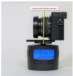
Again, the idea is to set the lens axis to be on the same rotational axis as the TurnsPro unit. I hope to do some field tests of both the iPhone and the GX80 soon.
