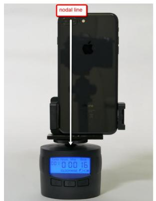
So, I designed a new mount which would set the iPhone 8 cameras on the correct axis for rotation.
