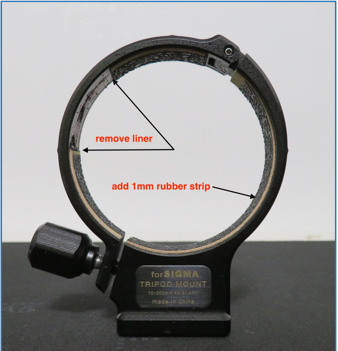
the completed mount
