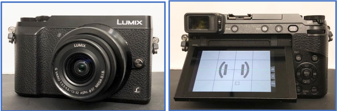
This is my Panasonic Lumix GX80 (GX85 in USA) fitted with the collapsible 12-32mm f3.5-5.6 lens
