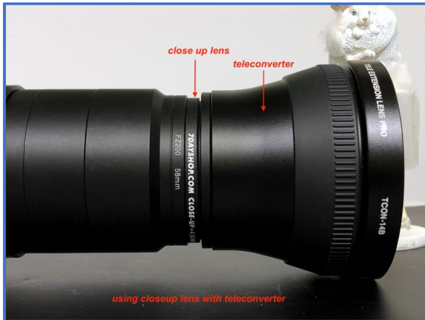
The TCon 14 (1.4x magnification used with adaptor tube on FZ300/330. A 58mm +4 supplementary lens is attached between the converter and the adaptor tube.
