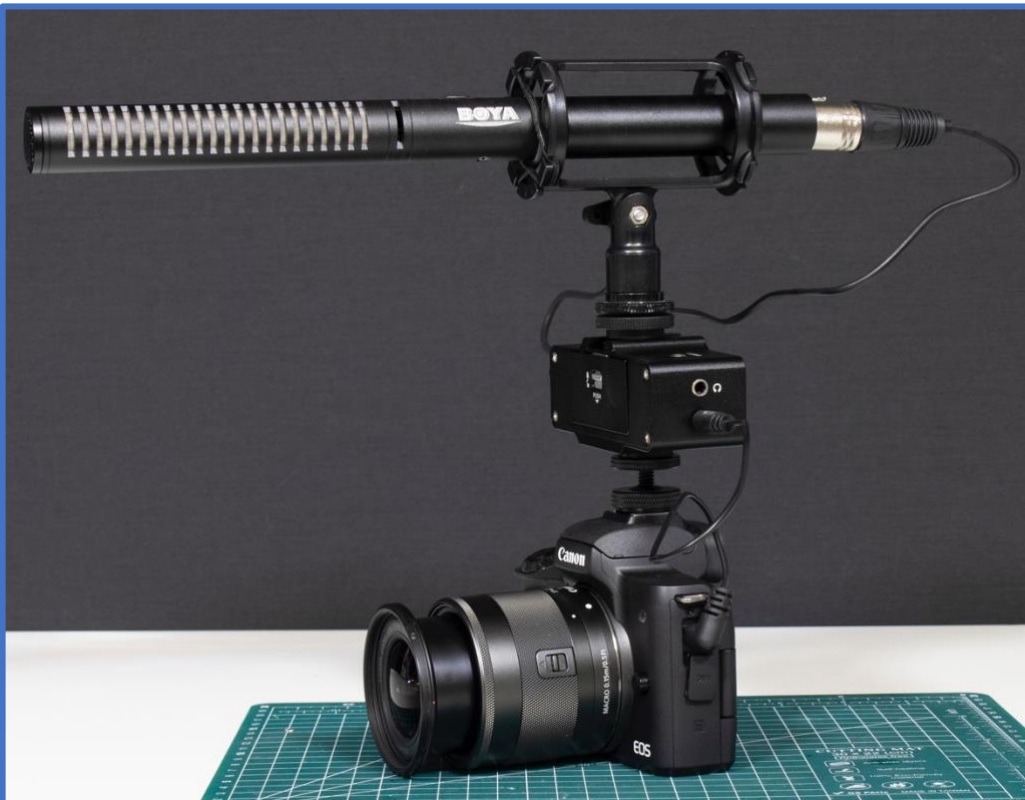
In this illustration, the BOYA BY-1000 Mic is used with the pre-amp.
