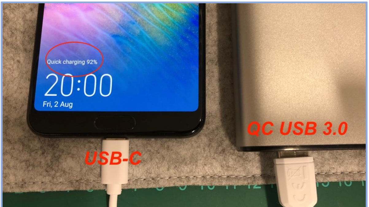
Similarly if a USB-C device is connected to a USB-3.0 QC (quick charge) port again the smartphone will negotiate quick charging.
