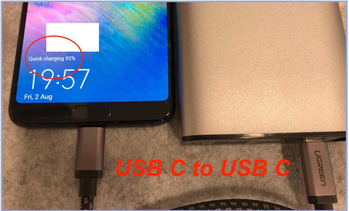
USB-C to USB-C (PD) connected smartphone and power bank showing the Quick Charging has been selected.
