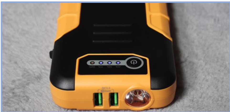
The two USB 3.0 QC ports on the unit each up to 3A
