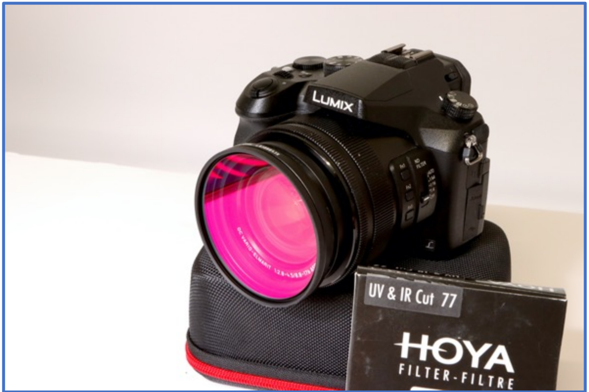
The Hoya IR + UV cut filter. Note the reflected colour of the filter.
