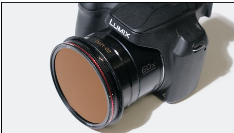
The modification allowing the use of my 72mm Freewell variable ND filter on the FZ82
